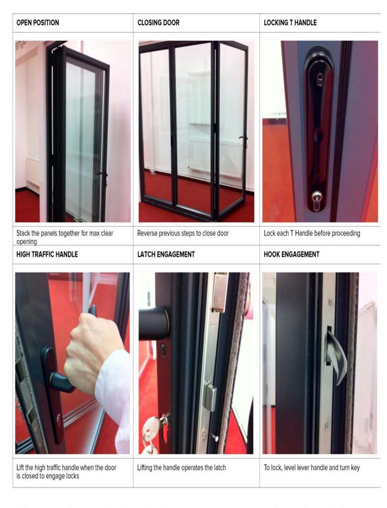
Failure to correctly operate the folding sliding door system can cause damage to the operating mechanism and hardware. This can cause the door to fail.
